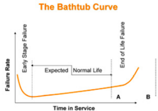
Figure 1: Bathtub curve representing a typical failure rate vs. time in service
