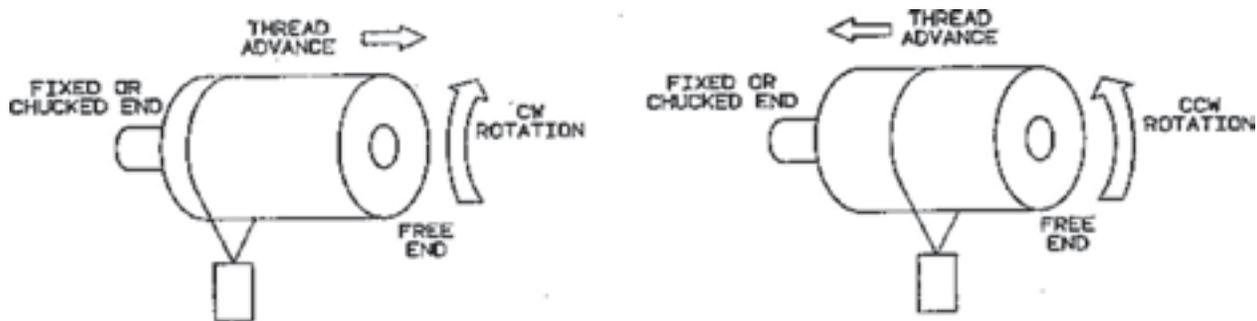
2. CCW or left hand lead: The thread will advance from the fixed or arbor end of the shaft towards the free end when the shaft is rotating counter clockwise (CCW). The thread will move from the free end of the shaft towards the fixed end for clockwise (CW) rotation. See B below.
